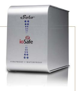
loSafe's technology protects disk drive data from damage from fire, floods and other disasters, while simultaneously resolving the heat dissipation issues found in all computer systems. Air-flow cooling helps dissipate heat during normal operation, and ioSafe's technology also can detect destructive heat levels and automatically close the vents to protect data from extreme heat.
